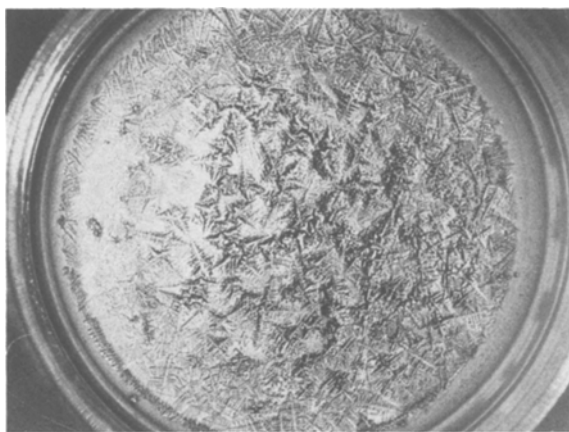
Fig. 4 Total view of a 0.5 mm-layer of gelatine plus 3% NaCl. The methylene blue stained layer is completely desiccated and NaCl crystallized within the network of the former cell structures. Direct photo of a petri dish under illumination from below
